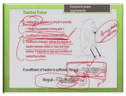
So, another important thing to be noted is weight on the power running gear of the machine. So, in common equipment or the common wheels of the cars whatever we are using, you can see that all the wheels of the car are not driving wheels. Common machines you can see that all the axles are not powered and all the wheels are not driving wheels. So, only some of the axles will be powered and the other axels will be just acting like a steering component.
