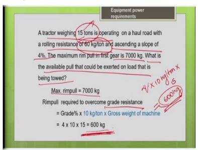
Now let us workout the problem on how to estimate the power requirements of the machine. So, a tractor weighing 15 tons is operating on a haul road, the gross weight of the machine is given as 15 tons. It means it includes it is empty weight as well as the load it is carrying, with the rolling resistance of 60 kg per ton, it is given you can take it from the literature also for this particular haul route.
