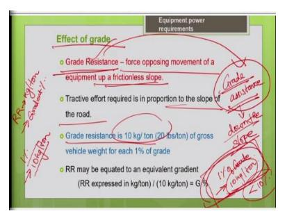
Grade resistance is nothing but by simple elementary I mean a mechanics people have worked out this the relations. Say for example, for 1% of grade so the amount of tractive effort needed to overcome this 1% of grade it is 10 kg per ton. So, this is simple guideline which they are worked out which is worked out in the literature you can easily find it. So, for 1% of grade, so the grade resistance is 10 kg per ton.
