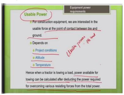
So, where a tractor is towing to load, the power available for towing can be calculated after detecting the power required for overcoming the various resistance forces from the total power. So, this we have to keep in mind, so this is nothing but your usable power.
