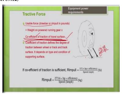
So, how to calculate this usable force? So, this usable force is going to depend upon the traction of your travel surface. So, as I told you how much amount of the total power becomes usable, it depends upon the degree of traction between your wheel and the ground. Traction is nothing but
