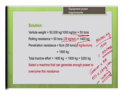
So, let us convert the vehicle weight into tons, because your rolling resistance is commonly expressed as kg per ton. So, let us convert the weight of the machine into tons you know that the gross weight of the machine is given as 50,000 kg. So, 1000 kg = 1 ton, so divided you will get the gross weight of the machine as 50 tons. Now the rolling resistance you need to calculate for this particular haul route it is given as 28 kg per ton.
