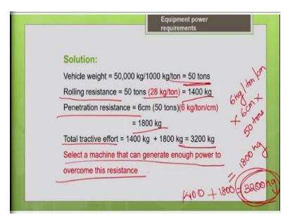
So, you multiply that by how much is the depth of penetration? It is nothing but 6 centimeter, and what is the gross weight of the machine? It is nothing but 50 tons. So, that gives you the penetration resistance as 1800 kg. Now we can find the total resistance, that is nothing but add your rolling resistance and the penetration resistance. It is nothing but your 1400 kg + 1800 kg, so that gives me the answer as 3200 kg is the total resistance.
