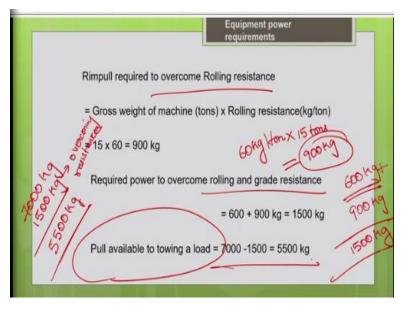
Now let us calculate how to estimate a tractive effort to overcome the rolling resistance? So, it is nothing but for this particular haul route the rolling resistance value is given us 60 kg per ton. So, what is the gross weight of your machine? It is nothing but 15 tons. So, that gives me the total
